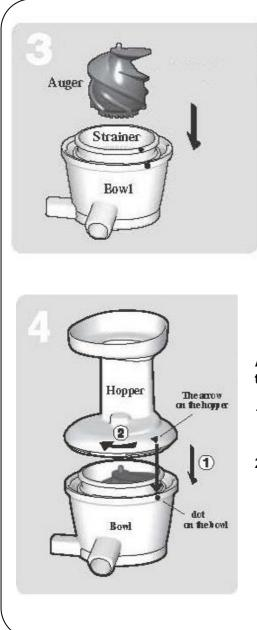
Push in the auger into the strainer
