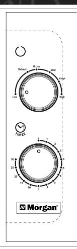
The control panel consists of two function operators. One is a timer knob, and the other, a power knob.
